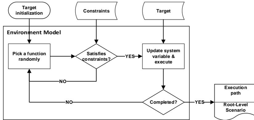
Figure 5: Scenario generation process for random testing
