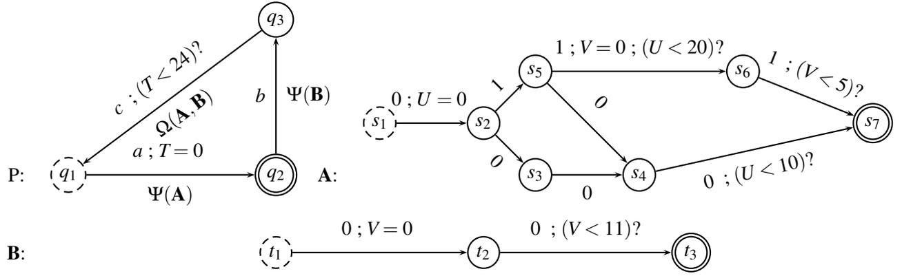
Figure 4: Parallel timing system  $S_3$ .  $\Delta_A = 25, \Delta_B = 11$ .
