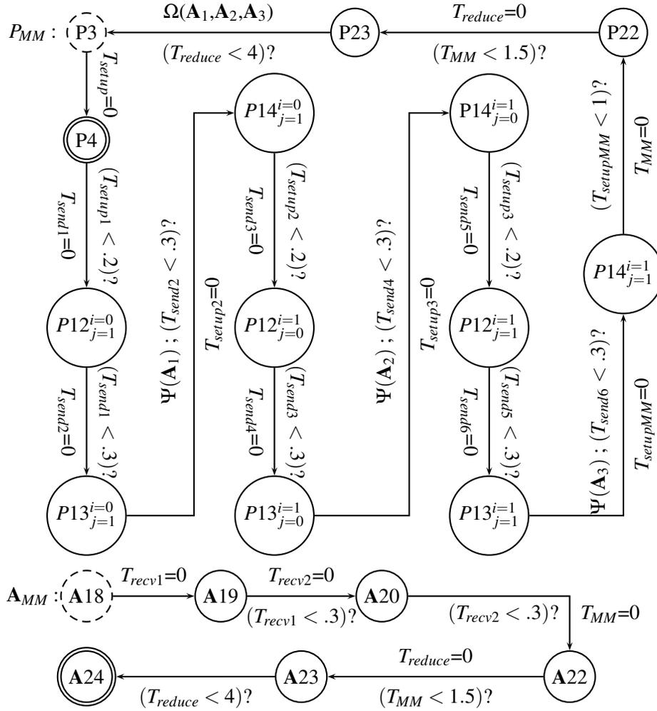
Figure 7: Parallel timing system  $S_{MM}$  for Algorithm 1 across a four processor cluster. Events have been elided for the sake of clarity. Upper bounds on timer constraints correspond to delay measurements taken over our implementation; times are given in milliseconds. Minimal variance from these bounds is ensured to the extent provided by the underlying RTOS.
