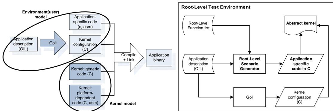
Figure 6: Root-Level scenario and the testing environment
