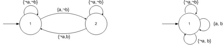
Figure 1: CCSL constraints: (a) a alternatesWith b (b) a subClock b
