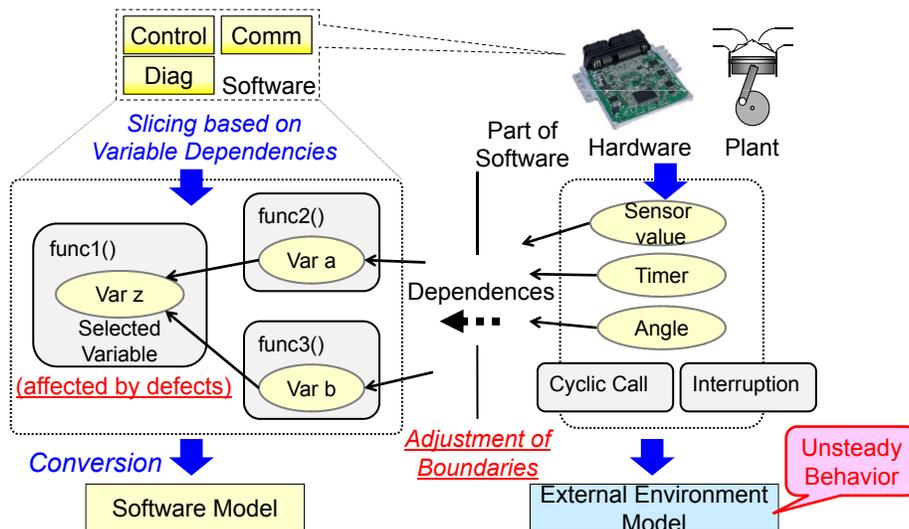
Figure 1: Modeling Method for Embedded Control System
