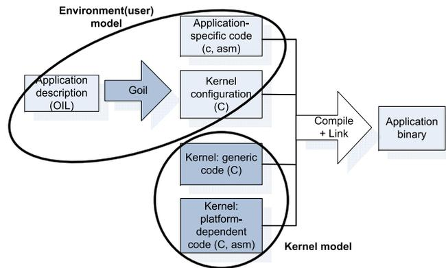
Figure 1: Components of Trampoline
